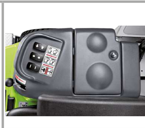
Controls via electric buttons
