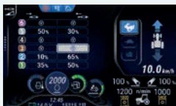
Electrohydraulic remotes flow set up
