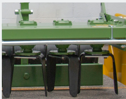
Wide spaced bearings on rotors
