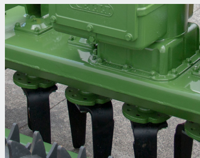
Fully welded gearbed
