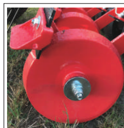
Press wheel has independent mount so always improves seed to soil contact.
