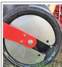
New depth gauge wheel for both open and closed operation depending on soil types, etc.
