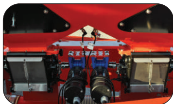
Single shot seed and fertiliser distribution system
